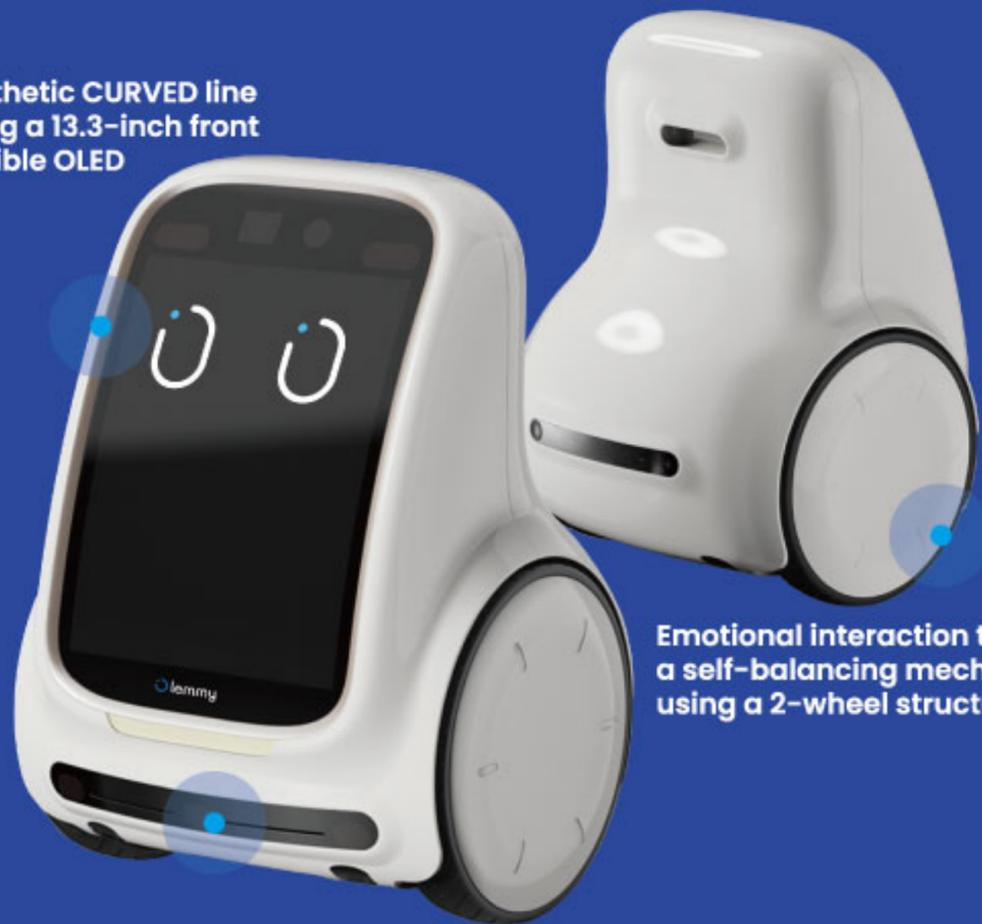
Emotional interaction through a self-balancing mechanism using a 2-wheel structure
